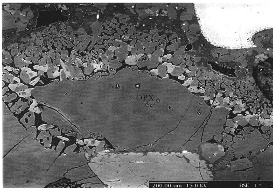
Fig. 1. Back-scattered electron image of orthopyroxene being replaced by fine-grained mineral assemblage.
